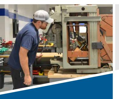
Trip Shaft Bearing Replacement in GE Magne-Blast Medium Voltage Breaker
